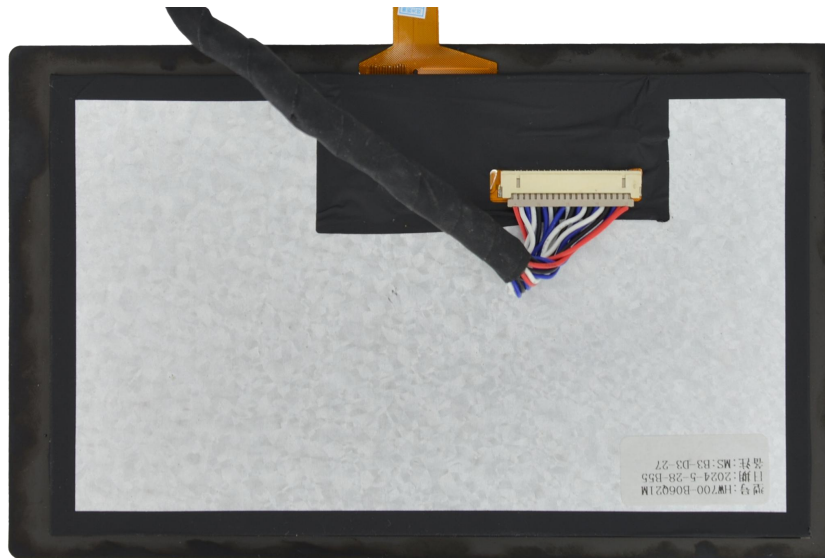
Figure 26 Connect LVDS screen cable to LVDS screen
